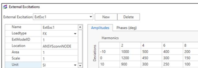
Also for the mechanical response analysis: external forces (forces that are not the pulsation-induced forces or cylinder stretch forces as calculated by PulsimSuite) can now be created with an **External Excitation** editor, which allows you to specify harmonic excitation force amplitudes and phases in a spreadsheet (copy from Excel is possible). You can also specify whether the force acts on a PulsimSuite node, or on a location in an external model.
