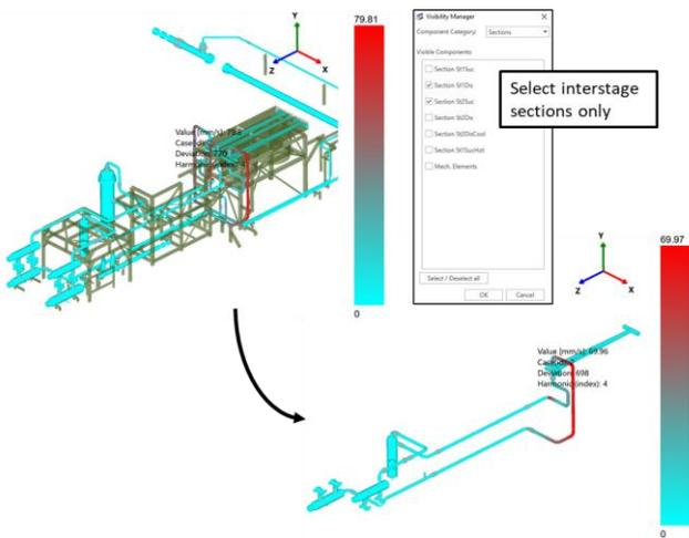
A new functionality in PulsimSuite is the option to hide parts of your model. This can be useful during the modeling of complex systems, and especially during the analysis of pulsation or mechanical results. With the **visibility manager**, you simply select the parts (Sections, Groups, Lines) of the model that you want to analyse, and the rest of the model will be hidden. The function that calculates the maximum response will only take into account the visible part of the model, of course.
