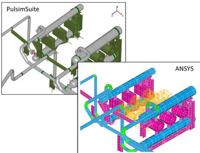
Although the functionality was already available for advanced users, the inclusion of **external mechanical models** and **external excitation forces** in mechanical simulations has been made much more intuitive, by GUI support. For this purpose, the GUI has two new tabs: One for the definition of your External Models (their names), and one for the definition of your **Mechanical Excitations**.
