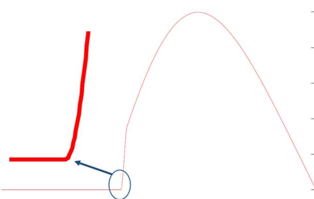
For pump systems, the flow pulse shape now represents the inertia of cylinder valve and liquid, at the moment when the cylinder valve opens. This greatly improves the convergence and stability of calculations for liquid systems. By faster convergence, the simulations have also become faster.
