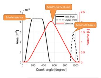
A new module in PulsimSuite is the **screw compressor** (SC node). With this optional module, you are able to simulate the pulsations generated by a screw compressor, by specifying its characteristics, see the picture to the left.
