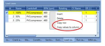
In all "bottom tab" windows that specify operating conditions, load cases, etc., you can now copy a full row, or copy a value from one of the boxes into all rows in that column. These functions can be found under the right-mouse button.
