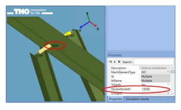
Joints (JNT) now have a master (and implicitly a slave) node definition: the MasterNodeID property. You can thus create e.g. several hinge connections to one structural location. Several JNT's can be connected to one Mechanical node, if that Mechanical node is specified as MasterNodeID.
