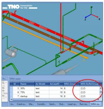
To reduce the calculation time of mechanical responses (by disregarding parts of a system in the mechanical runs), PulsimSuite 2.2 introduced the "MRA group".
